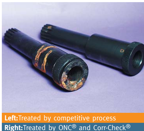
Left: Treated by competitive process Right: Treated by ONC ® and Corr-Check ®
